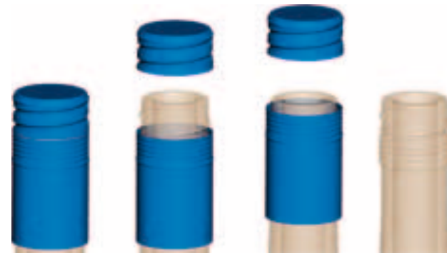
Full recycling of aluminium: studies to remove the aluminium skirt
